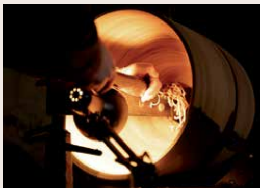
Meredith’s vessels are hollowed from unseasoned oak to as thin as 1/8" (3mm) in preparation for the cutting and folding process.
