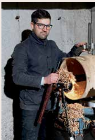
Meredith’s vessels are hollowed from unseasoned oak to as thin as 1/8" (3mm) in preparation for the cutting and folding process.
